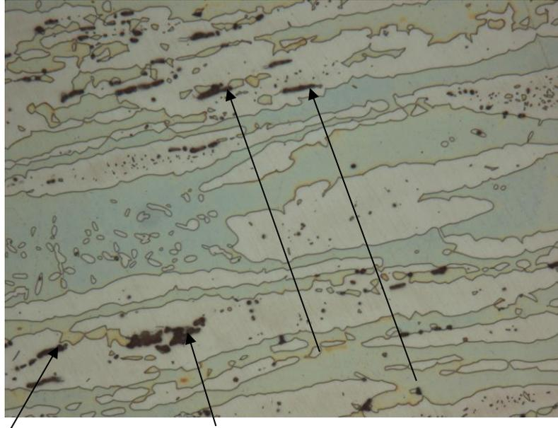
These dark patches within the microstructure (taken at x500) are signs of "Sigma Phase", which is detrimental to Super Duplex
