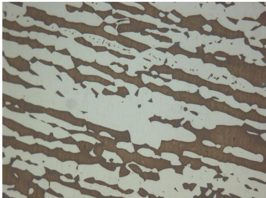
The above microstructure, taken at the same magnification, is free of sigma phase and any other detrimental aspects to Super Duplex
